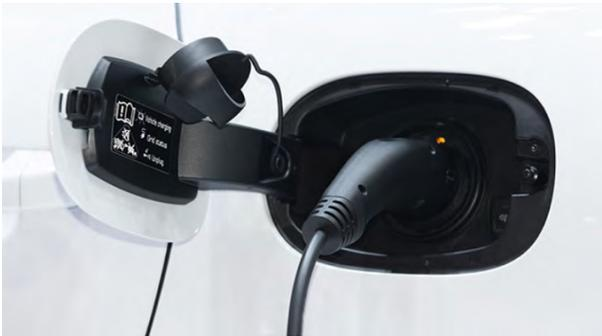
Figure 2-7. Level 2 Electric Vehicle e-Charger
